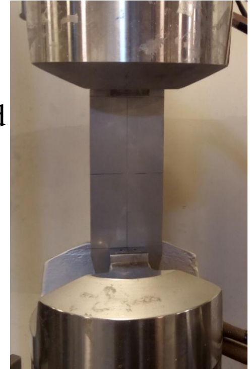
Fatigue test for crack generation
