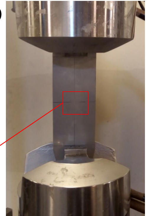
Fatigue test for crack generation
