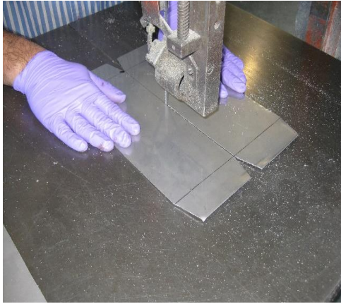
Cutting the specimen using horizontal band saw
