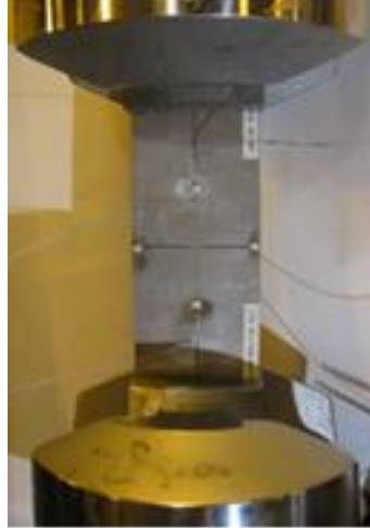
Figure 2. Specimen mounted on the MTS machine for fatigue pre-crack generation
